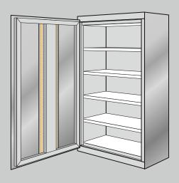
A reliable bonding joint of metal stiffener and frames in metal bodies can be achieved with Sikaflex® -545 with fast
