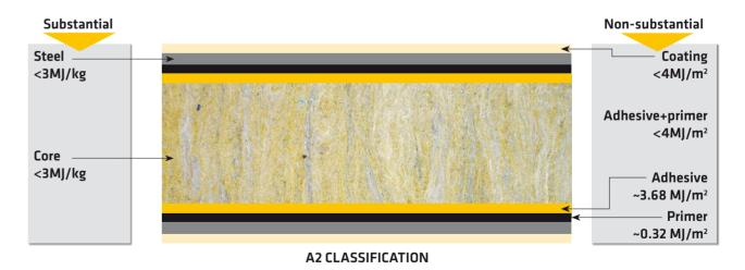
Classification A2 is one of the highest achievable ratings for an insulated bonded panel and Sika has solutions that customers use to achieve A2, s1, d0 classification on their panels.
