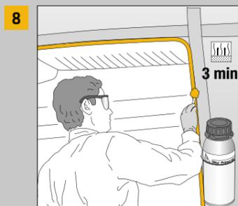
8 ■ Using a brush apply a thin continuous coat of Sika® Primer-207 on the damaged area and let it dry for a minimum of 3 minutes
