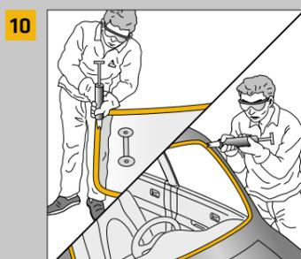
10 ■ Using a triangular nozzle apply the adhesive on the glass or on the body
