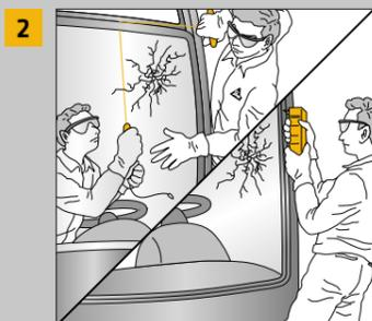
2 ■ Cut out damaged windshield using electrical knife, cutting wire, cold knife, etc.
