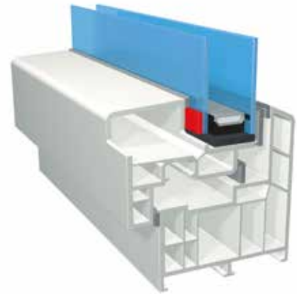
Interior Overlap Bonding with Sikasil® WT Technology
