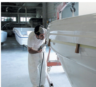
Sealing with Sikaflex®-295 UV
