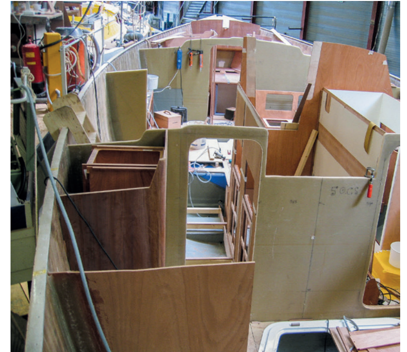
Lightweight panels being fitted to an open hull
