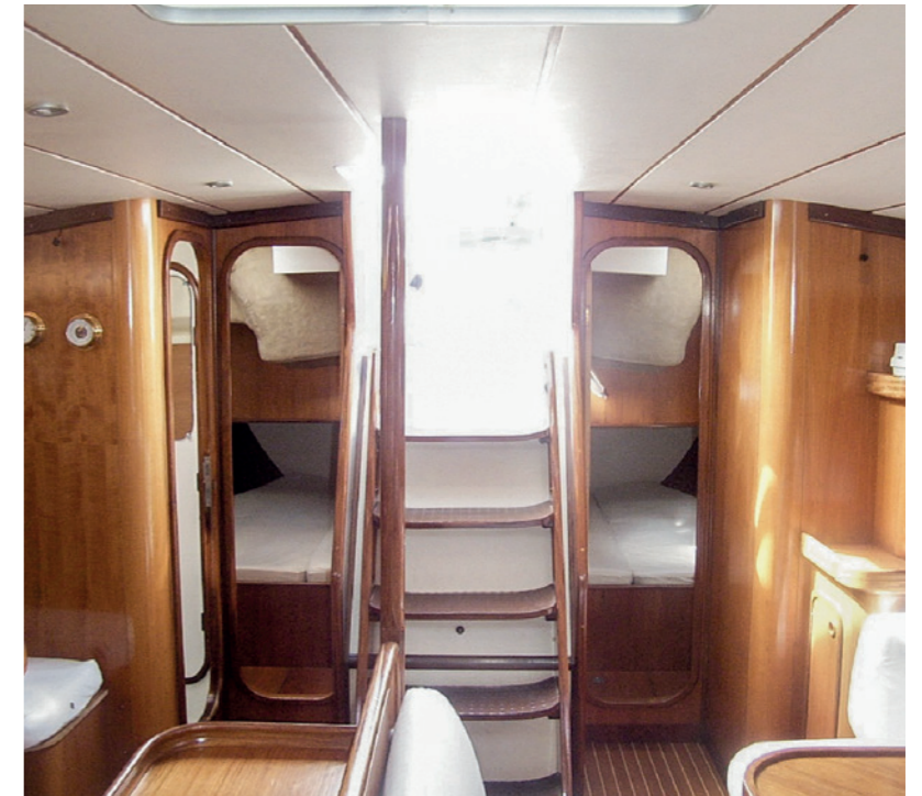
High-quality lightweight panels finished in traditional high-gloss wood veneer and bonded using Sikaflex®-292i
