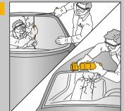
■ Cut out damaged windshield using an electrical knife, cutting wire, cold knife etc.
