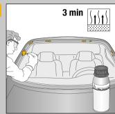
■ Cover any minor damage to paint work using Sika® Primer-207. In case of larger areas contact your body shop or refer to the car manufacturer's specification
