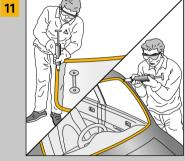
■ Apply a triangular bead of adhesive either to the glass or the aperture
