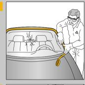
■ Cover the aperture with masking tape
