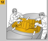
■ Place the windshield in position within the open time of the adhesive
