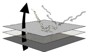
Sports and outdoor clothing consists of two to three laminated layers. This multilayer set-up includes an outer fabric, a lining fabric and a membrane between them. Our SikaMelt® adhesives are the ideal solution for various kinds of membranes like PTFE, PU and PES. Properties such as low viscosity, fast curing and a long shelf life are especially developed to increase your productivity.
