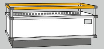
Structural bonding and sealing of organic glass on metal frame with **Sikaflex®-260 N**. For applications requiring food approval, **Sikaflex®-522** can be used for sealing or Sikaflex®-551 for sealing and bonding. Reliable assembly of displays and small components in plastics and metals with **SikaFast®-5215 NT**. Body removable sealing with **SikaLastomer®-710**.
