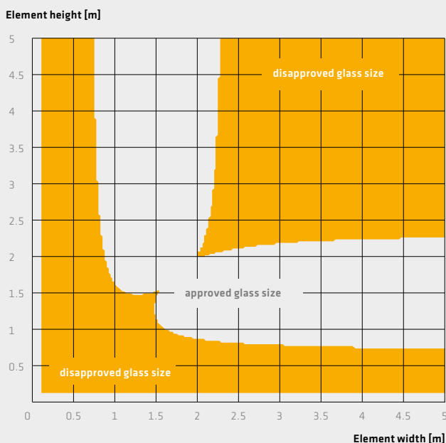
Fig. 4a: Feasible triple glazed IG unit with Sikasil® IG-25 and the same conditions as in Fig. 4b IG configuration 8/10/4/10/8 IG Joint dimensions 10 mm x 6 mm
