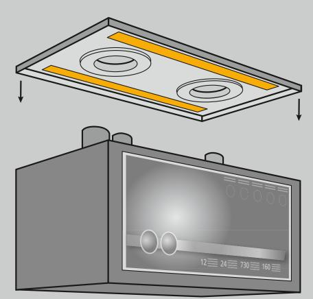
Top lid bonded and sealed with SikaMelt®-9670.
