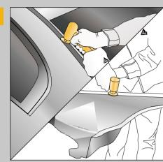
■ Grind bonding areas on both car body and new panel to bare metal
