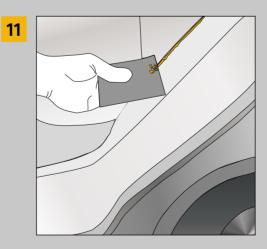
■ Tool any adhesive squeeze-out to seam along the bonded edge
