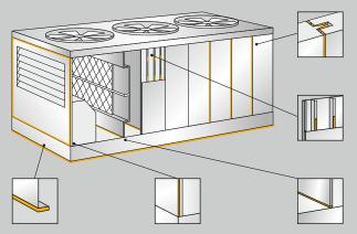
Elastic structural bonding and sealing of metal frame and body in heating, ventilation and air conditioning systems can be achieved with Sikaflex®-551 with ultimate mold and fungus resistance.
