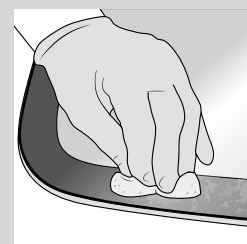
3 rd step: Use 1 fresh unit Sika® Cleaner PCA. Start cleaning ceramic frit
