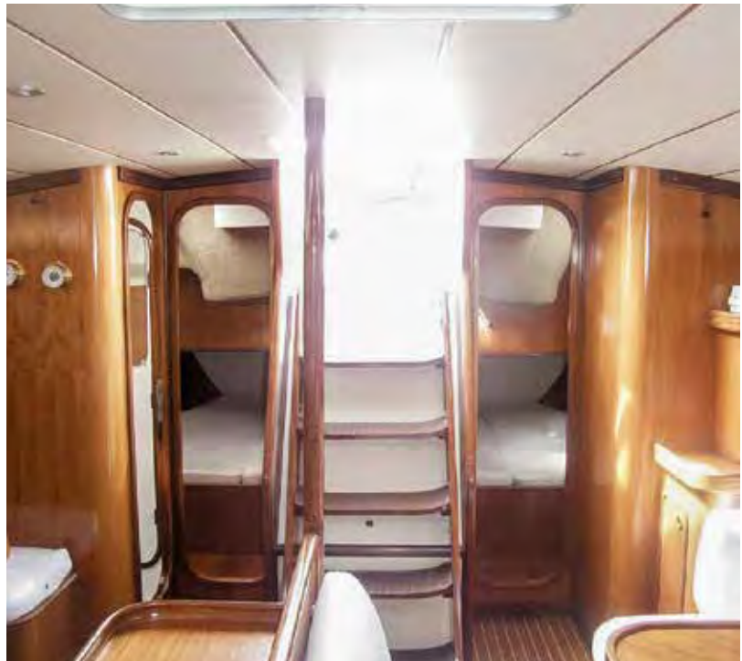
High-quality lightweight panels finished in traditional high-gloss wood veneer and bonded using Sikaflex®-292i
