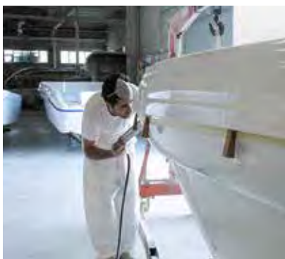
Sealing with Sikaflex®-295 UV
