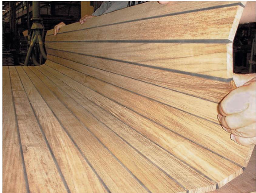
Fig. 16 Deep joint prefabricated teak decking and the strength and flexibility inherent in the adhesive
