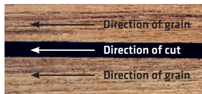
Fig. 22 Always ensure that the direction of cut is with the grain to avoid 'digging-in' damage to the sides of the planks
