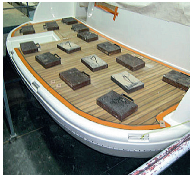
Fig. 20 Holding in place with weights
