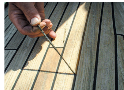
Fig. 34 A triangular cut of the old caulking being removed manually
