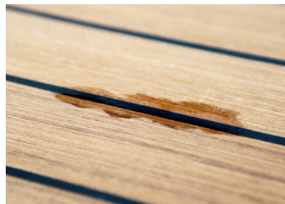
Fig. 21. Discolouration of the wood is a tell-tale sign of a failed or damaged joint in this teak deck
