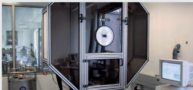
Impact test machine with pendulum (ISO 11343) for velocities of 1 m/s to 5 m/s at temperatures from -50 to 80 °C. As glass deforms with a max. speed of 4 m/s, this is the optimal range for simulating bomb blast tests.
